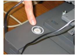
The base power switch is located near the back, on the right hand side; turns on film light
